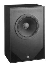
Screen Sub IA provides low distortion, true sub-bass response for any cinema environment. Built with a shallow profile, like the Screen 4 and Screen 5, the sub is designed for behind-the-screen placement. The unit uses a single 18" (460mm) long excursion high power driver. Large area tapered twin ports ensure minimum turbulence down to the lowest frequencies demanded by today's digital sound tracks.
